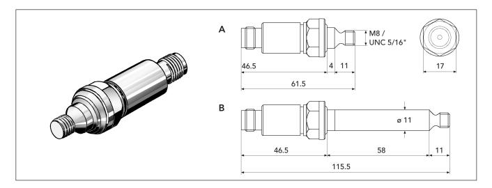
Standard shock pulse transducers are used in all permanent SPM installations for bearing monitoring. They are installed in countersunk mounting holes on the bearing housings.
